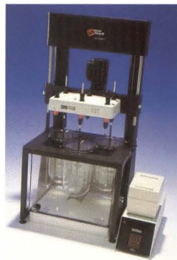
Figure 4: Hanson 4-Liter Dissolution Test Station
