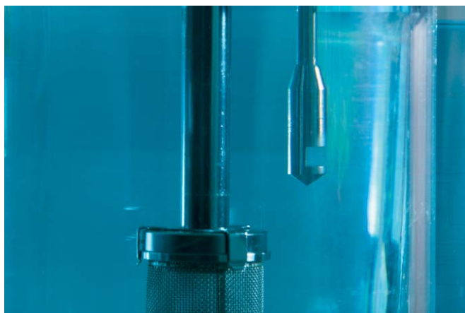
Figure 1: A fiber optic probe allows measurements of dissolved product contents directly in the dissolution vessel. The probes come in a variety of shapes, sizes and orientations depending on the vendor source.
