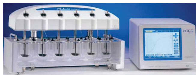
Figure 1. Fiber-optic drug dissolution in situ test system.
