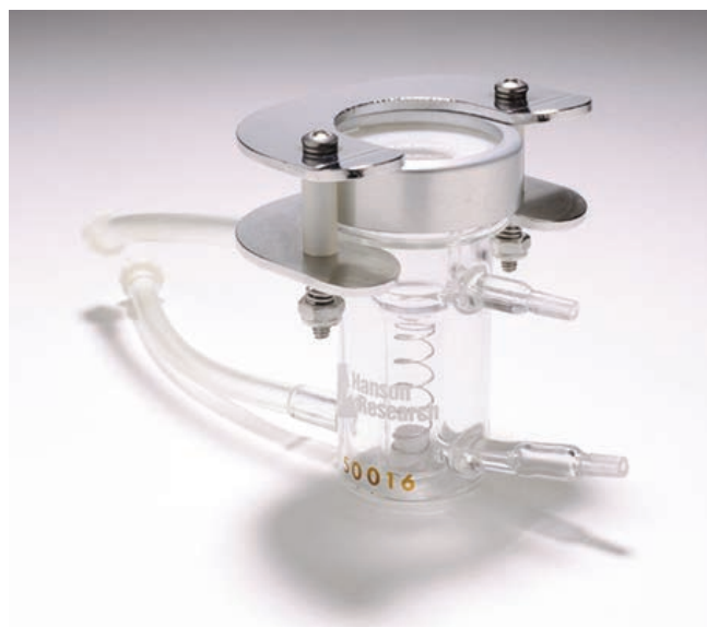
Figure 1. Vertical diffusion cell (VDC) assembly.
