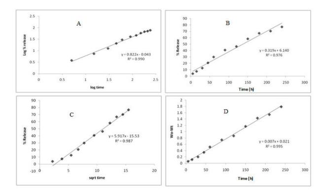
Figure 7. Graphical presentation of in vitro drug release data according to (A) Korsmeyer, (B) zero-order, (C) Higuchi, and (D) Hixson-Crowell models.
