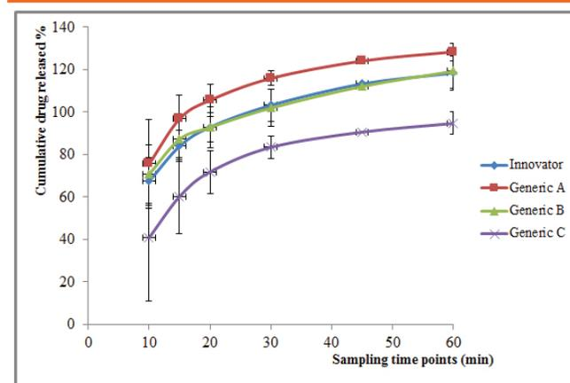
Figure 3. Cumulative dissolution profiles of selected amoxicillin (500 mg) products at pH 6.8.
