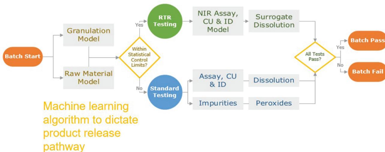
Figure 11. Real-time release using a "health check" model to evaluate current batches against a historical standard. RTR: real-time release; NIR: near infrared; CU: content uniformity; ID: identity.
