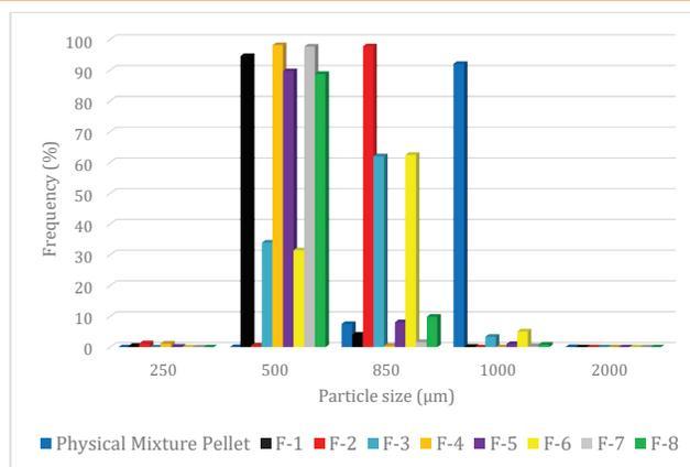
Figure 2. Particle size distribution of hydrochlorothiazide formulations.
