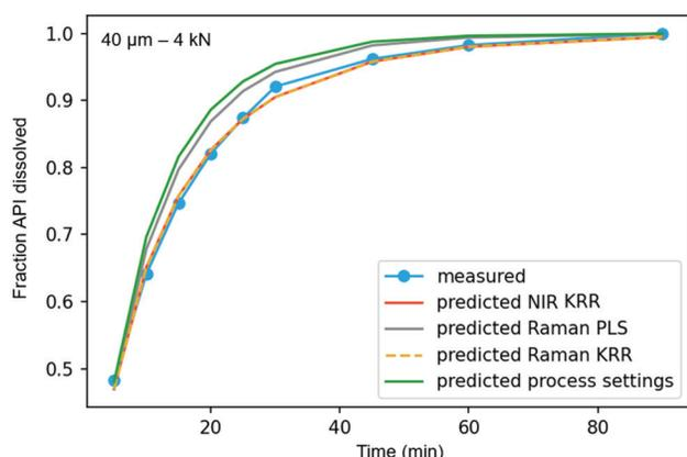
Figure 5. Representative example of the predicted and measured dissolution profiles for a tablet with an API particle size of 40  $\mu\text{m}$  compressed with 4 kN. API: active pharmaceutical ingredient; KRR: kernel ridge regression; NIR: near infrared; PLS; partial least squares.
