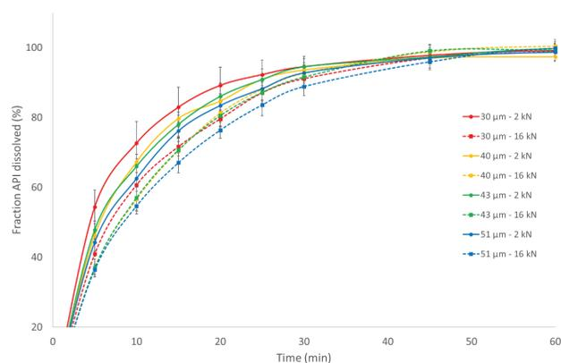
Figure 4. Dissolution profiles of tablets compressed with the lowest (solid line) and the highest (dotted line) compression force for the API batches with differing particle size. API: active pharmaceutical ingredient.
