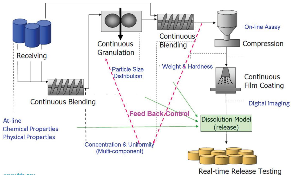
Figure 6. Example of real-time release testing within a continuous process, wherein input materials are continuously received into the system with continuous blending, granulation, compression, and film coating followed by parallel at-line and inline assays.
