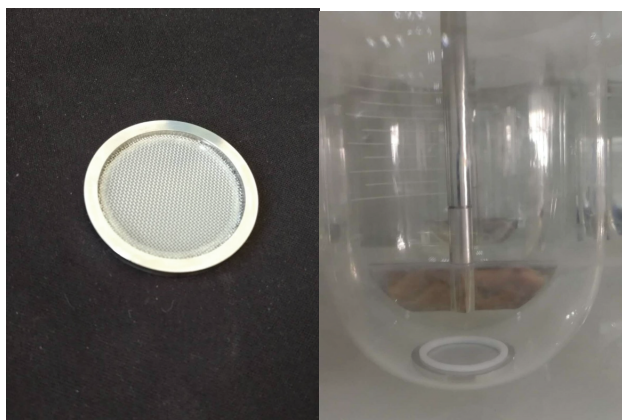
Figure 1. Photograph of USP Apparatus 5 (Model: UST-814, Logan Instruments Corp., Somerset, NJ, USA).
