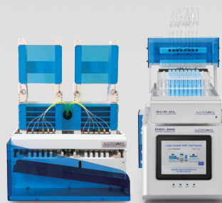
Filter changer for collection of samples for offline HPLC analysis
