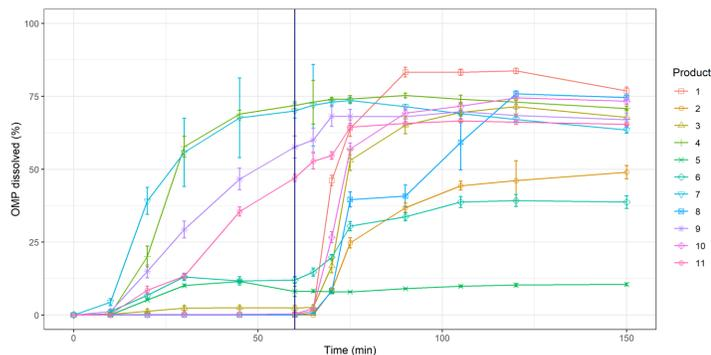
Figure 4. Dissolution profiles of 11 multi-source omeprazole products in the multiple dose scenario (MDS). Blue line indicates the addition of the neutralizing buffer at 60 min. Values are mean  $\pm$  SE.
