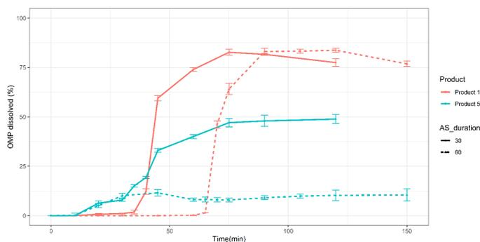
Figure 5. Dissolution profile of products 1 and 5 shows the impact of gastric residence time under the multiple dose scenario (MDS). AS: acidic stage duration (30 or 60 min).
