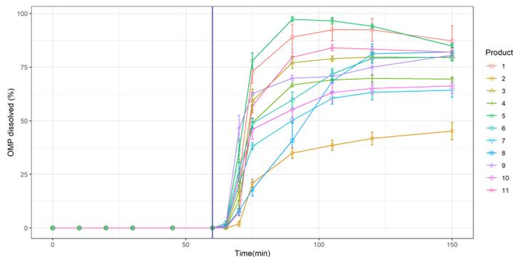
Figure 3. Dissolution profiles of 11 multi-source omeprazole products in the single dose scenario (SDS). Blue line indicates the end of the acidic stage by addition of neutralizing buffer at 60 min. Values are mean  $\pm$  SE.
