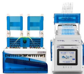
Filter changer for collection of samples for offline HPLC
