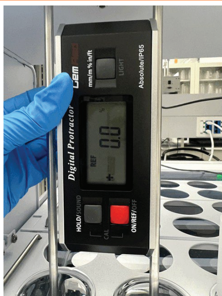
Figure 3. Electronic level to determine shaft verticality of apparatus 3.
