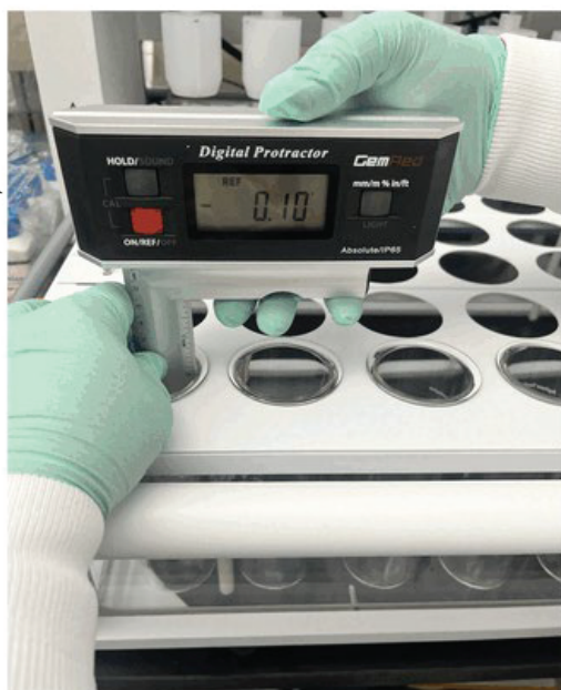
Figure 4. Measurement of apparatus 3 vessel verticality.
