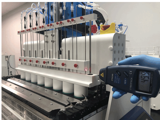
Figure 5. Digital measurement of the reciprocation rate. (Printed with permission of Logan Instruments).
