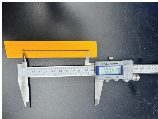
Figure 8. Measuring stroke distance with a calibrated caliper.
