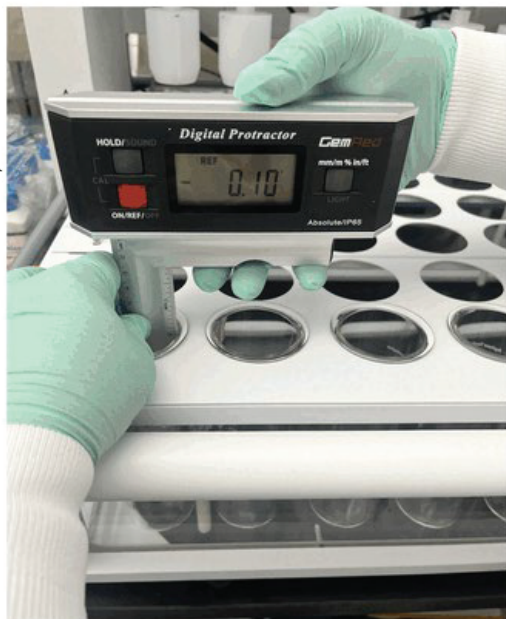
Figure 4. Measurement of apparatus 3 vessel verticality.
